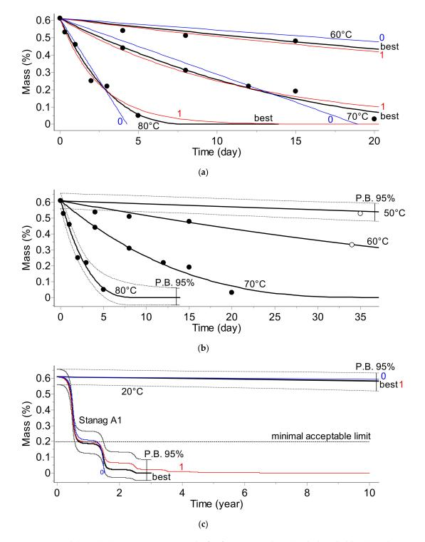
**Figure 3.** Stabilizer depletion (UPLC) test. (**a**) The fit of experimental data by the best (bold), 0th, and 1st order models. (**b**) Prediction of the long-term reaction course for temperatures of 80, 70, 60, and 50 °C (predictions are verified by experimental data marked as empty circles). (**c**) 10-year predictions for 20 °C and climate category STANAG A1.
