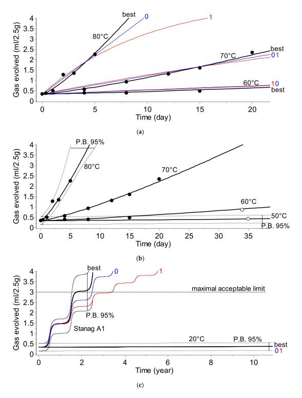
**Figure 2.** Gas evolution (VST) test. The plots present: (**a**) The fit of experimental data by the best (bold), 0th, and 1st order models. (**b**) Prediction of the long-term reaction course for temperatures of 80, 70, 60, and 50 °C (predictions are verified by experimental data marked as empty circles). (**c**) 10-year predictions for 20 °C and climate category STANAG A1.
