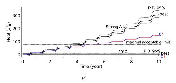
**Figure 4.** Heat evolution (HFC) test. (a) The fit of experimental data collected at 90, 80, and 70 °C by the best (bold), 0th, and 1st order models. (b) Prediction of the long-term reaction course for temperatures in the range of 90–50 °C. The predictions for 60 and 50 °C are verified by experimental data marked as empty circles collected once a year. (c) 10-year predictions for 20 °C and climate category STANAG A1.
