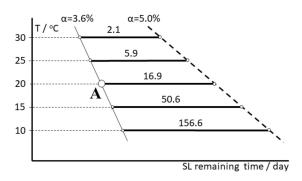
**Figure 12.** Dependence of the shelf life (SL) remaining time on the isothermal temperature which allows the prediction of the usability of the sample stored at 20 °C with a deterioration progress of 3.6% (point A). The remaining values of the shelf life at temperatures between 10 and 30 °C are displayed in days on the thick horizontal lines.
