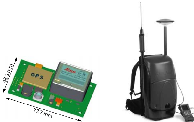
Figure 4: Pedestrian Navigation System (PNS) (left) developed together with Leica Vectronix. With a size of 73.7 mm x 48.3 mm x 18 mm and a weight inferior to 50 grams, it fulfills all ergonomic requirements for such application. Right, the POS/LS™ (Position and Orientation System for Land Survey) system of Applanix for high precision surveying.
