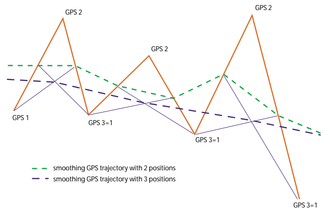
Figure 4: two different ways to smooth the GPS trajectory in order to compute a precise GPS azimuth and correct the misalignment of the PND.
