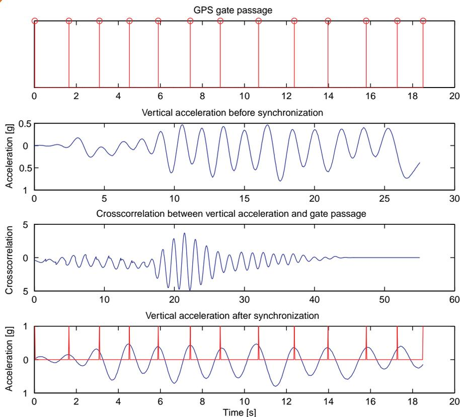
**Figure 3.** The vertical acceleration helps determine at which moment the skier bends down to pass a gate and when he or she stands up again. Coupling this information with InMotion Technologies's video shots provides a powerful and complete tool for run analysis.
