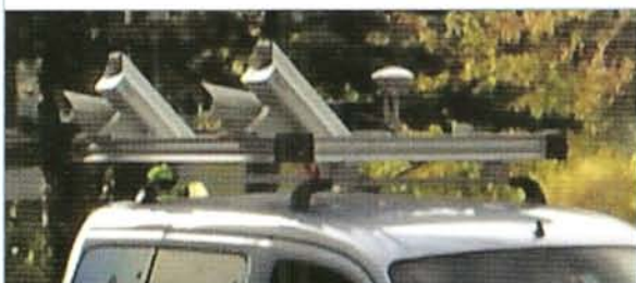
Figure 8 : Cameras mounted for building capturing
