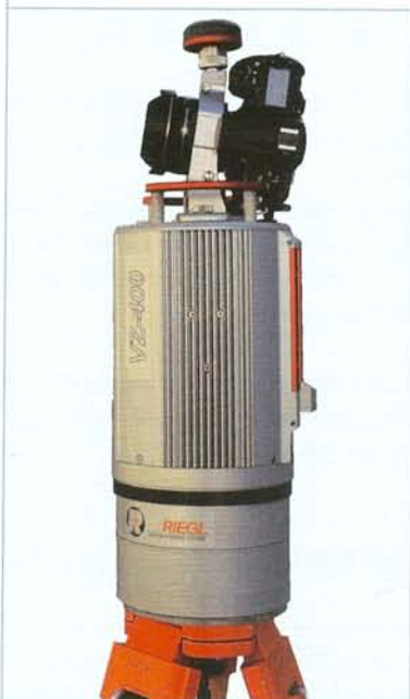
Figure 2 : Riegl VZ-400 laser scanner with Nikon D700 digital camera
