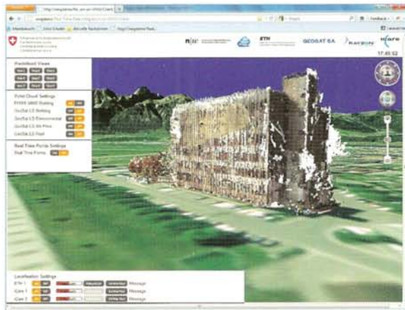
Figure 5 : Continuous Location Demonstrator application with point cloud of building acquired by stereo vision mobile mapping system
