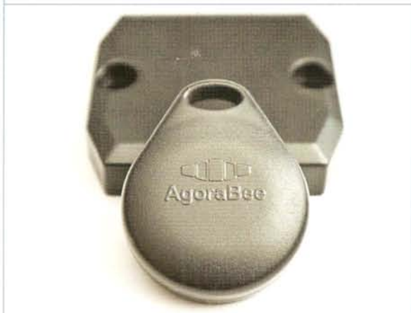
Figure 13 : RFID active tags used for simultaneous friend-foe identification and localization.
